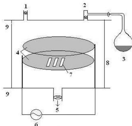
**Fig. 2:** Plasma polymerization setup: 1. Pressure gauge, 2. Monomer inlet through a flowmeter, 3. Monomer container, 4. Steel plate electrode, 5. Vacuum pump, 6. AC power supply, 7. Substrates, 8. Glass cylinder 9. Brass flanges.
