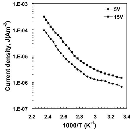
**Fig. 4:** Variation of current density with inverse absolute temperature for PPBMI thin film in the ohmic and non-ohmic regions (Thickness,  $d=150$  nm).
