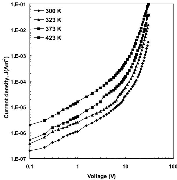
**Fig. 3:** Voltage dependence of current density for 150 nm thick PPBMI thin film.
