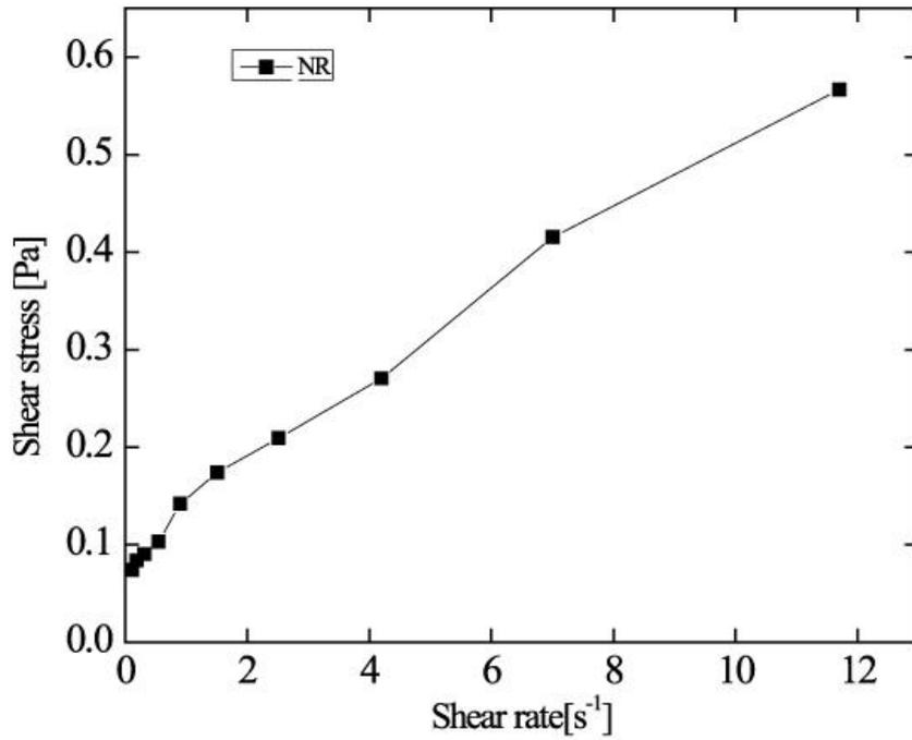
Fig. 7: Shear stress vs shear rate plot for NRL at 1% speed, 25<sup>0</sup>C and MV<sub>1</sub> system.
