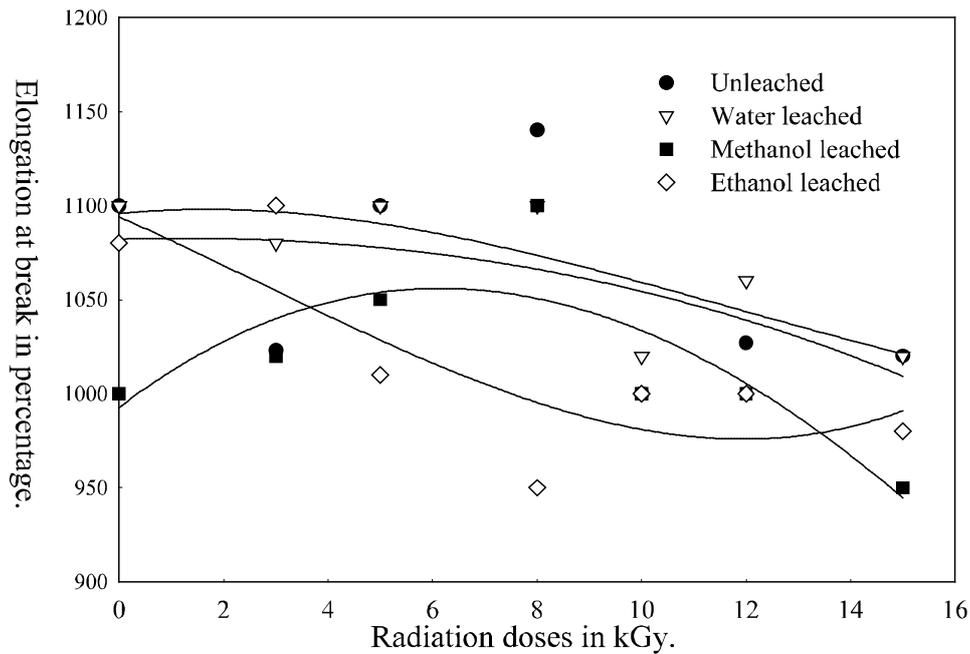
Fig. 6: Effect of radiation doses and leaching on elongation at break of NRL films.
