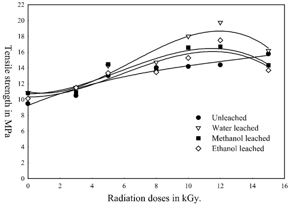
Fig. 5: Effect of radiation doses and leaching on tensile strength of NRL films.
