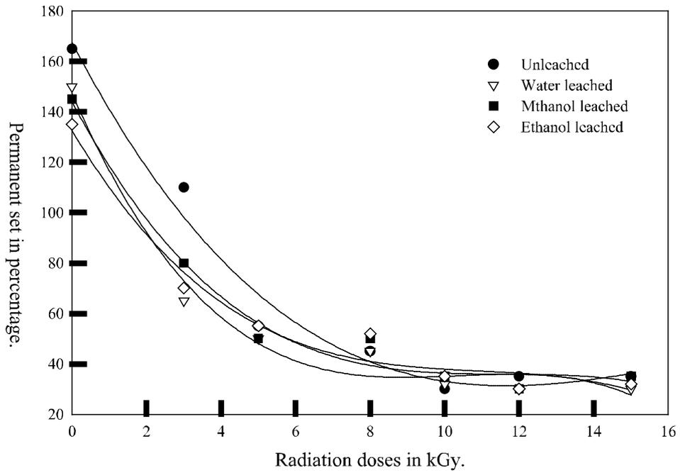
Fig. 1: Effect of radiation doses and leaching on permanent set of NRL films
