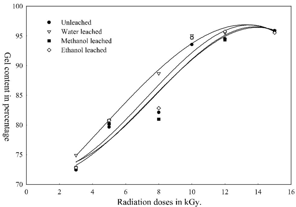
**Fig. 4:** Effect of radiation doses and leaching on the gel contents of NRL films.
