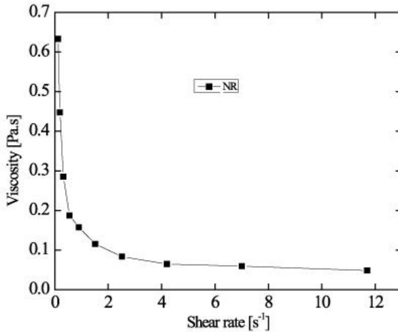
Fig. 8: Viscosity vs shear rate plot for NRL at 1% speed, 25<sup>0</sup>C and MV<sub>1</sub> system.
