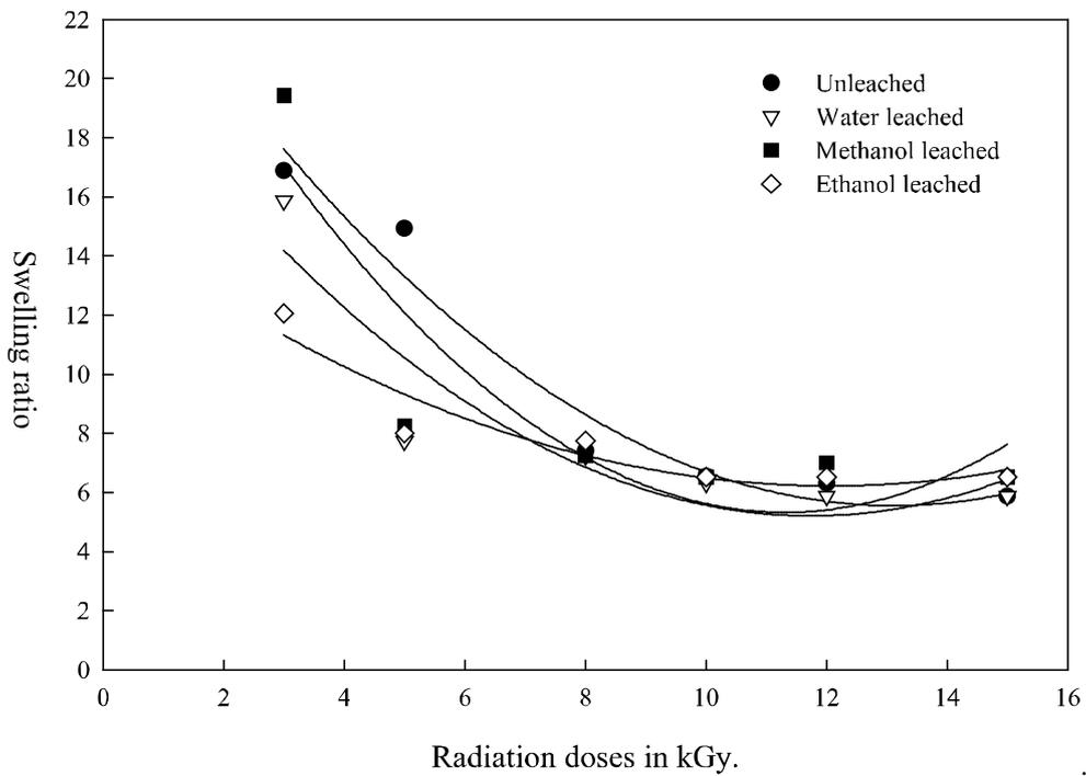
Fig. 2: Effect of radiation doses and leaching on swelling ratio of nrl films.
