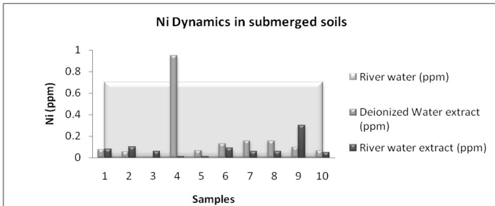
Fig. 2: Movement of Nickel in soil-water system
