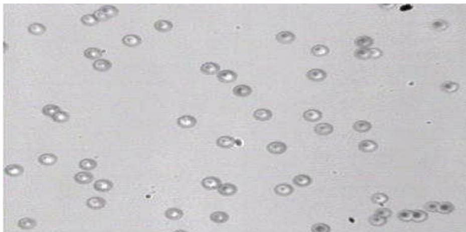
*Fig. 1: Tracks from alpha particle for ABS polymer*
